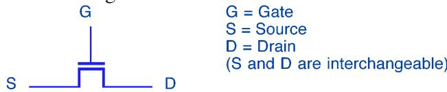
The NMOS transistor may be configured to operate in one of three different states, as determined by the **voltage** at the gate terminal  $V_G$ :
